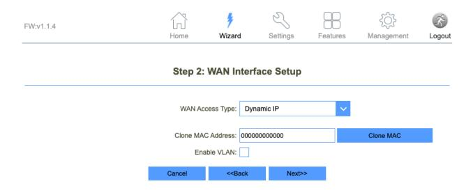
The WAN Interface Setup page is used to set the WAN Access Type.
